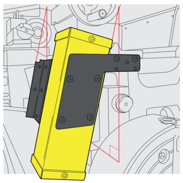
IT IS CRITICAL that the box is vertical & that the edge of the material is just touching the point at the bottom of the inverted V on the bed and it runs horizontally along the bed at right-angles to the box - B
